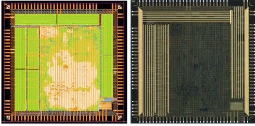
**Figure 2:** Layout (left) and die photo (right) of the TETRISC SoC
