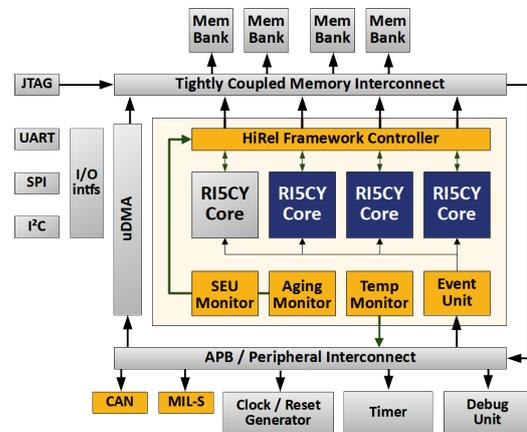
Figure 1: The system architecture of the TETRISC SoC
