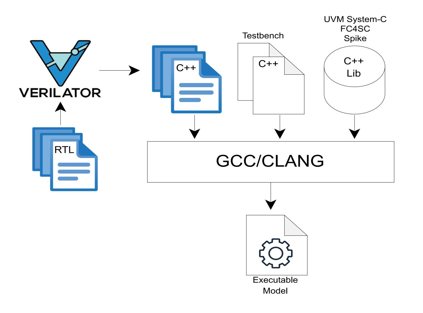
**Verilator:** an open-source tool that is able to transpile RTL code written in Verilog or SystemVerilog into a C++ model which can be instantiated in a wrapper along with the test bench code having as a result an executable containing the RTL functional model and its test bench.
