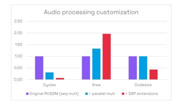
Then experiments were undertaken to add over 40 DSP custom instructions. This resulted in a core that ran the algorithm 14.3x faster than the original. The core was almost double the initial area but the codesize was 43% of the original.
