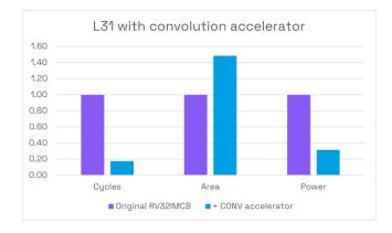
The modified L31 is 48.3% larger in area but has a throughput improvement of 5x and power improvement of 3x compared with the original L31.
