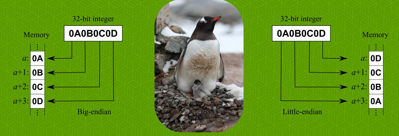
There are two (sane) standards for loading data in/out of CPU registers: little endian (LE) and big endian (BE). With LE, the data's least significant byte is stored in the smallest memory address and the most significant in the largest. It is vice versa for BE.
