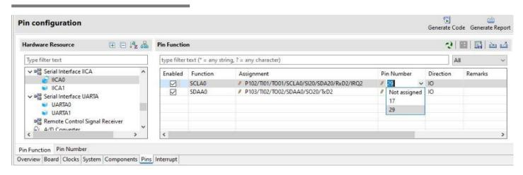
Display pin function options, assign pins per each peripheral module, check consistency and resolve pin multiplexing conflicts automatically
