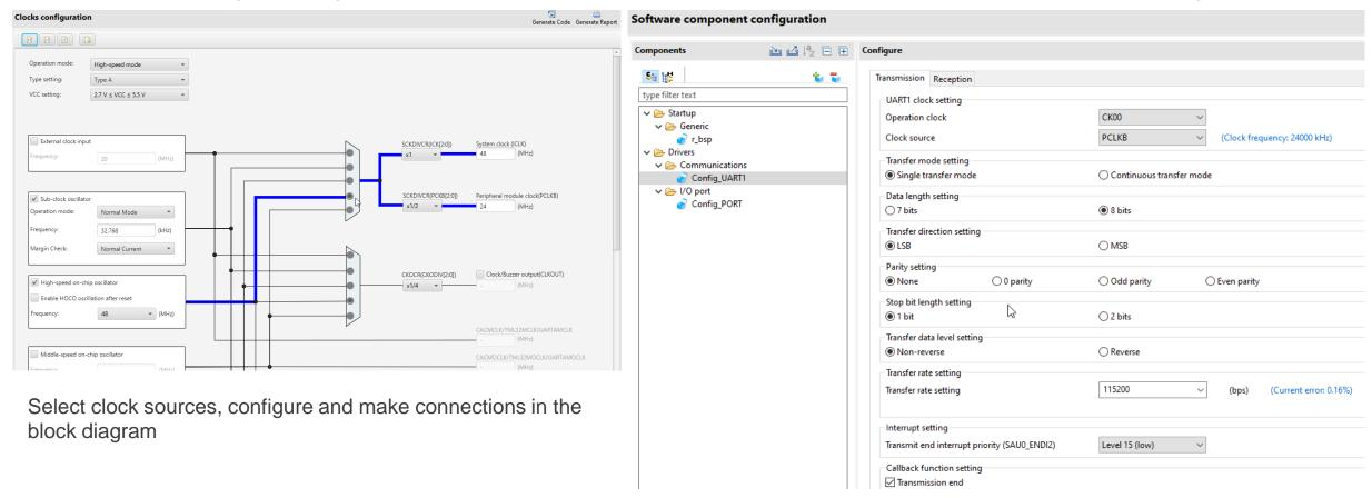
Add sw modules, setup peripherals, check for errors, switch the channels for use by drivers of multi-channel modules
