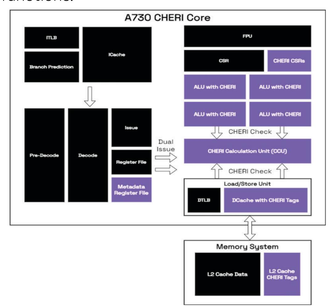
The register file, and some CSRs, are extended to 129 bits to accommodate capabilities. The memory system is extended to atomically handle capability tags while still using standard interfaces.
