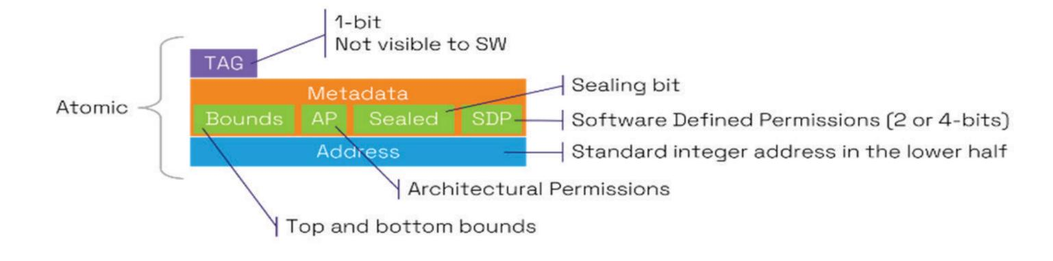
Integer-based memory pointers are replaced with capabilities to protect memory. For example, the Program Counter (pc) is a capability that grants permission to execute instructions from a constrained region of memory.
