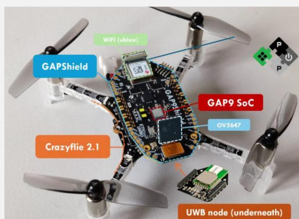
GAP9Shield[3] integrating the GAP9 SoC with 10 RISC-V cores. The shield and the UWB Loco Positioning Deck [4] are mounted on the Crazyflie 2.1 nano-drone [5].
