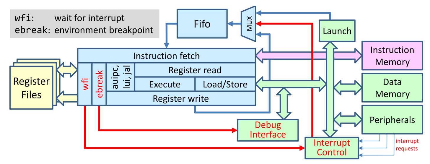
ebreak tokens flow to a debug interface and are handled by a debug server.
