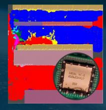
Rad-hard demonstrator with LEON5FT SPARC V8 32-bit processor and NOEL-V RISC-V 64-bit processor ST 28nm FDSOI GEO P2 technology
