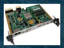
GR765 FPGA prototype on development board GR-CPCIS-XCKU115
