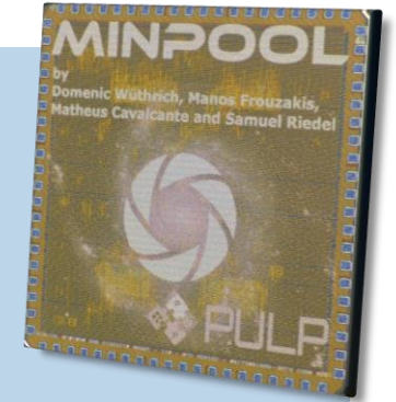
MinPool (2021) 16 cores, 200 MHz TSMC65, 2.4mm x 2.4mm
