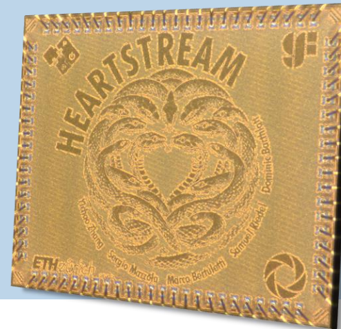
Heartstream (2024) 64 cores, 720 MHz GF12, 2.5mm x 2mm
