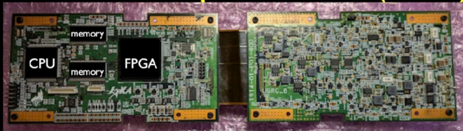
Initial version of LEV-I onboard computer board (used for radiation tolerance test)
